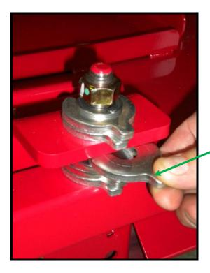
This photograph shows a shim that has been removed from above the bracket being reinserted below the bracket in order to increase the height of cut. Repeat this exercise for all three height adjustment brackets before attempting to tighten the adjuster shim retaining nuts.
