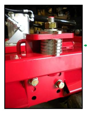
Once the shims on all three adjuster points have been moved to the desired position, tighten the retaining nuts firmly. *Do not leave them loose as this will cause the shims to fall out during operation.* This photograph shows the height range bolts selected to 'top left and middle right' with the shims arranged 'five below and one above. This will give a height of cut of 50mm as shown on the height decal.
