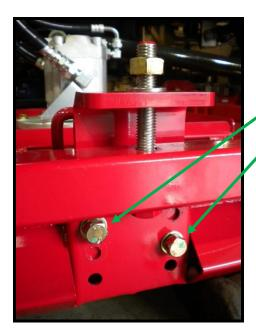
You can now see that the bolts have been inserted into their new position of 'top left and middle right'. If you refer back to the height chart decal you will see that this now puts this deck into the lowest range of 20 to 56mm.
