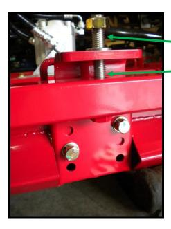
This photograph shows all of the shims removed from above and below the bracket. This should be done on all three units before proceeding.
