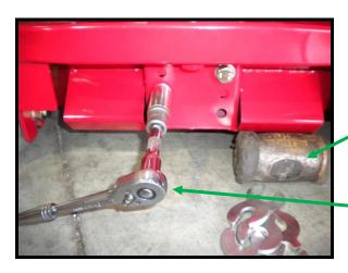
Support the deck underneath the bracket to be moved using a suitable item such as a mallet as shown.
