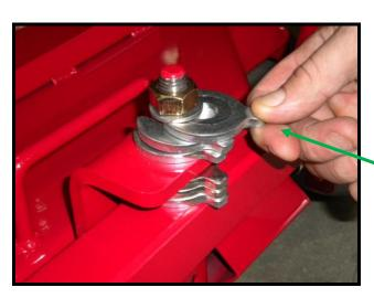
Once all three nuts are loose, remove shims in order to achieve the desired pattern as stipulated on the height range decal. If you need to increase the height of cut you will need to remove shims from above the bracket and replace them below the bracket. To decrease height, remove them from below the bracket and replace them above the bracket and replace them above the bracket.
