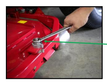
To adjust the height of cut, first of all loosen all three height adjustment s shim retaining nuts. It is important to loosen all three nuts at once and not try to adjust one bracket at a time. Trying to adjust one bracket at a time will make the task very difficult as it will have the effect of trying to twist the deck.
