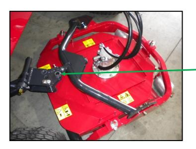
It is much easier to adjust the two rear units by swinging them out. In order to make this easier ensure that the removable pin is kept clean and greased. Periodic wire brushing of this pin prior to greasing will ease the removal of these pins. You will also find it easier to remove the pins and swing out the rear units if the machine is parked level ground.
