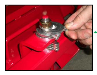
Remove all six of the shims from above and below the bracket.
